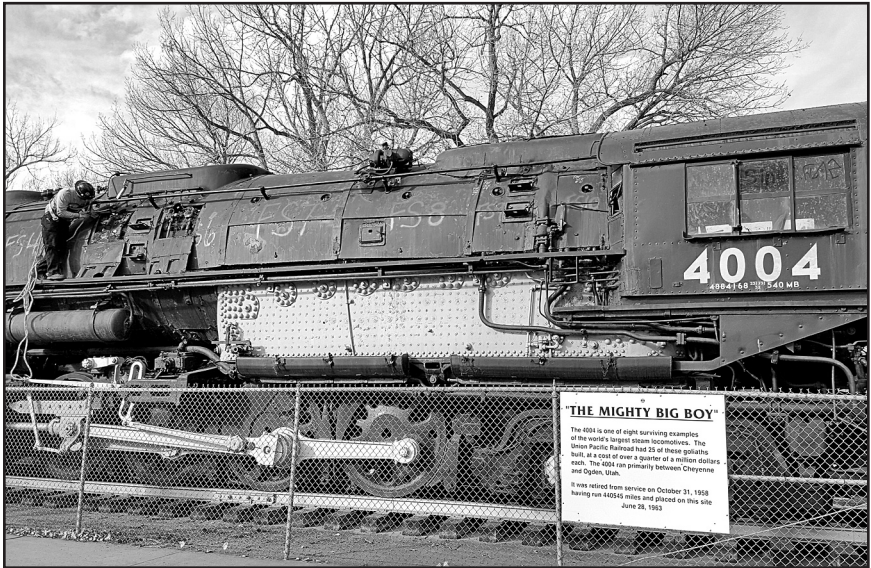
Preparation work in advance of asbestos removal on UP “Big Boy” 4004 at Holliday Park in Cheyenne, Wyoming. – Photo © 2018 Dave Schaaf.
